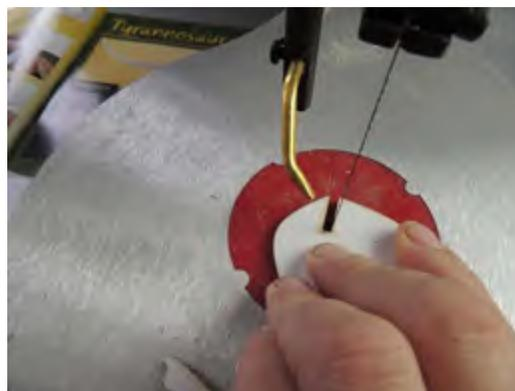
Always cut to the outside of the pattern line. Cutting to the outside will make the tab just a little too narrow, making the fit very tight. Cutting to the inside of the lines will make the fit too loose, making it necessary to re-cut the entire piece. Test fit the tab with a small piece of waste wood. If the fit is too tight, simply remove a small portion of wood with the scroll saw or with a piece of coarse sandpaper until the fit is perfect.
